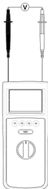
Figure 5 Voltage Measurement using test probes
