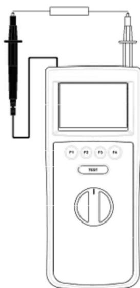
Figure 4 Earth Continuity/Insulation Measurement using Cordless probe
